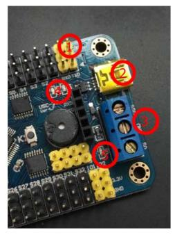
Servo power supply (+): VS (left of the blue connecting terminal at Position 3 in the figure)
