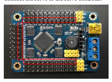
What is marked red in the figure are the servo's connectors for signal wires (be careful about the direction when connecting to the servo).
